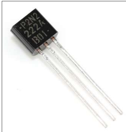
Figure 6-9: The small print on this transistor tells you exactly what it is.
