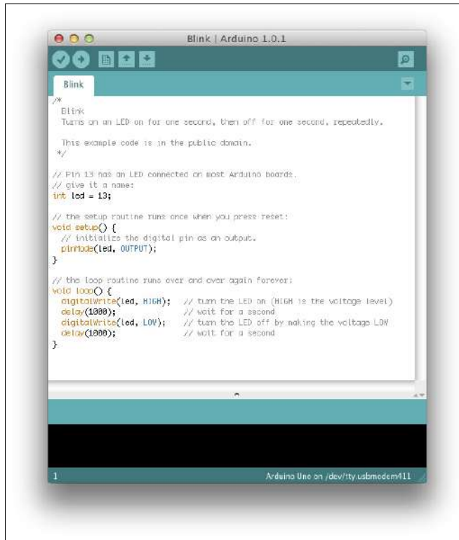
Figure 4-2: The Arduino Blink sketch.
