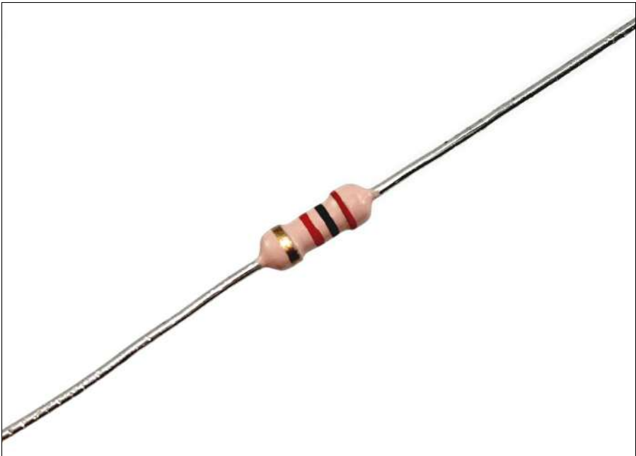
Figure 6-10: A close look at the color bands on a resistor.
