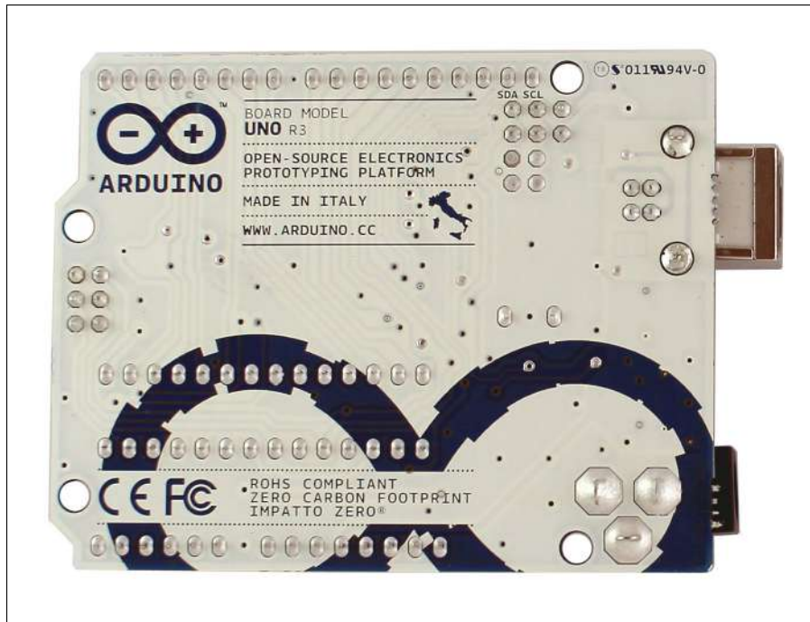
Figure 2-2: The back of an Arduino Uno R3.
