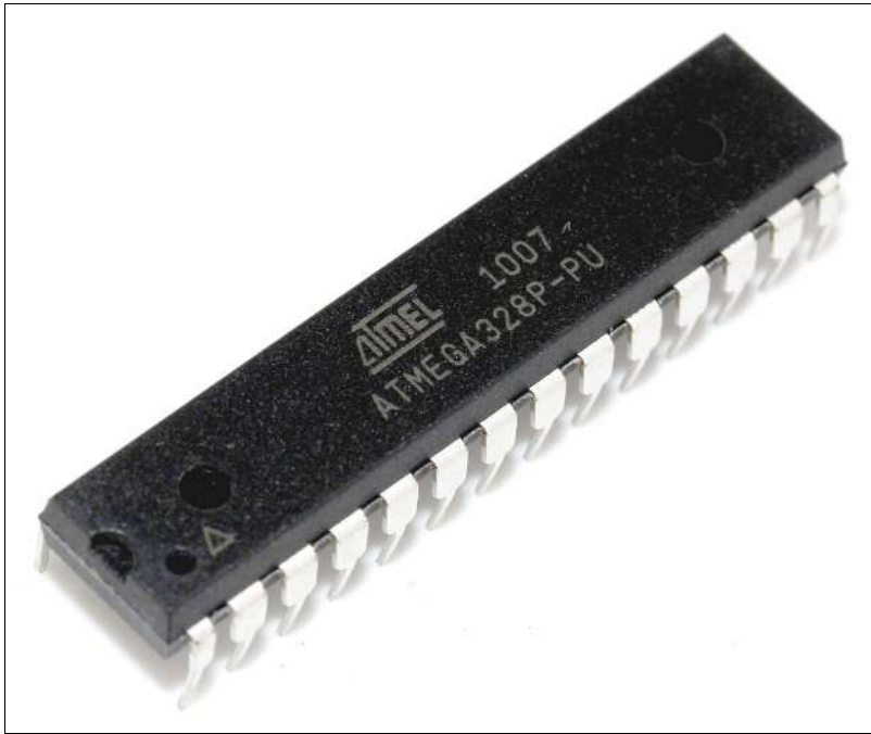
Figure 2-3: An ATmega328 microcon- troller all by itself.
