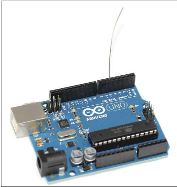
Figure 12-7: A photo of a DIY capaci- tive sensor.
